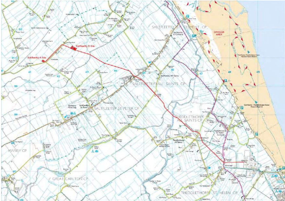
Figure 3 Saltfleetby Development Sites and Existing Gas Pipeline to (Decommissioned) Theddlethorpe Gas Terminal, Source Roc Oil
